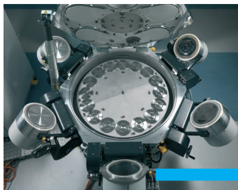
Figure 1. CLUSTERLINE® 200 system equipped with BPM with 4 sputter and 1 plasma source
