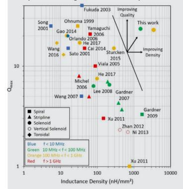
**Comparison of Magnetic Core On-Chip Inductors**
