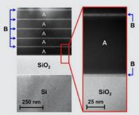
Figure 3: Cross-sectional Transmission Electron Microscopy (TEM) image of a soft magnetic multilayer sputtered on a Si/SiO<sub>2</sub> wafer in an Evatec batch tool. The dark contrast thick layers labelled with "A" represent the soft magnetic layers (e.g. CoTaZr, FeCoB, NiFe, etc.), whereas the light contrast thin interlayers labelled with "B" represent the dielectric interlayers (Al<sub>2</sub>O<sub>3</sub>, AlN, Ta<sub>2</sub>O<sub>5</sub>, SiO<sub>2</sub>, Si3N<sub>4</sub>, etc.).
