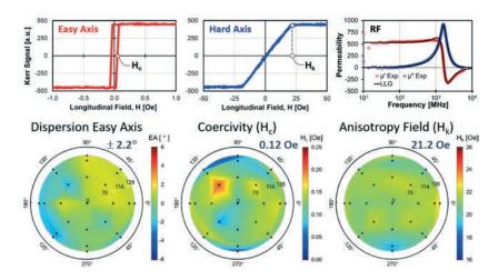
Figure 5. Results on 300mm depicting the static and dynamic magnetic properties of a several micrometers thick CoTaZr/Ta<sub>2</sub>O<sub>5</sub> multilayer.
