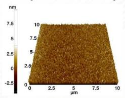
Figure 4. 10um by 10um AFM topography of an AI0.8Sc0.2N film deposited on Mo bottom electrode: the surface is free of abnormal grains.
