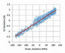
Figure 1. Deviation from average of the coupling coefficient as a function of Al0.7Sc0.3N thin film stress variation: the slope is steep and translates into 0.5% of coupling change every 50 MPa
