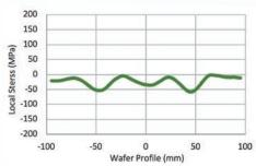
Figure 3. Within-in-wafer stress profile for an Al0.9Sc0.2N film deposited with the optimized process. The stress range is below ±50 MPa up to 5mm E.E.
