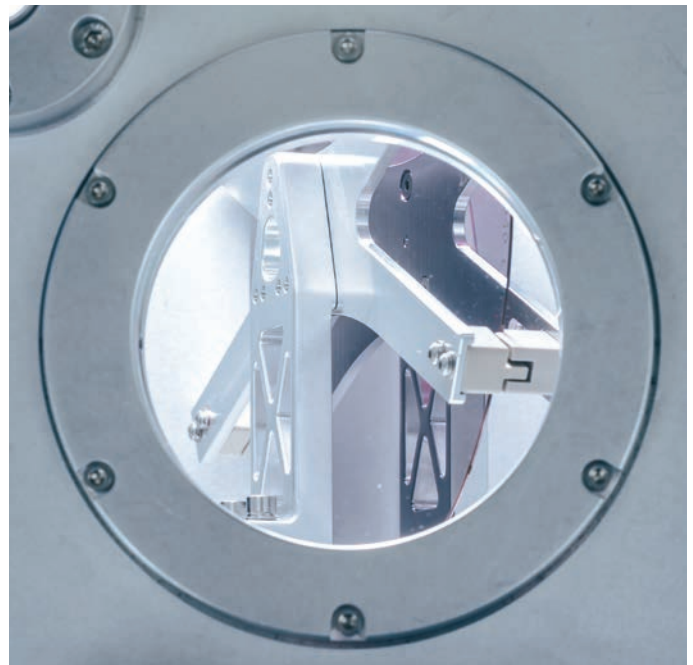
In-situ substrate flipping for double sided filters and stress control
