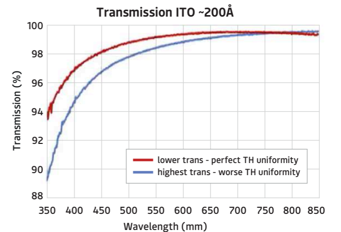
Figure 3b: Typical transmission performance for a thin ITO
