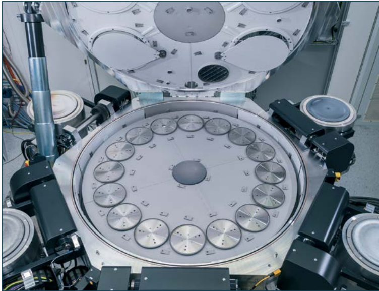
The latest generation of CLUSTERLINE® 200 BPM integrating a turntable with individual rotating chucks, proprietary cathode magnet technology and in-situ broadband monitoring.
