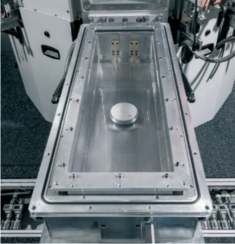
Integrated plasma source enables precleaning or new coating process options
