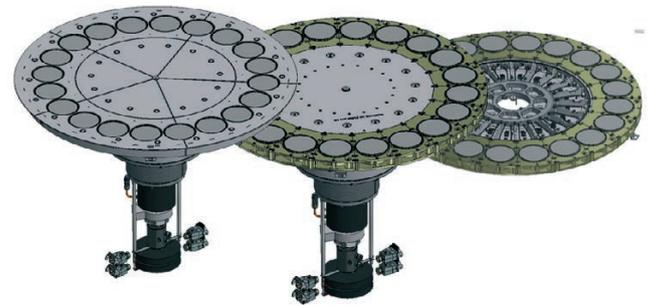
Concept of the hot ITO turntable with individual chuck segments and its cooling supply.
