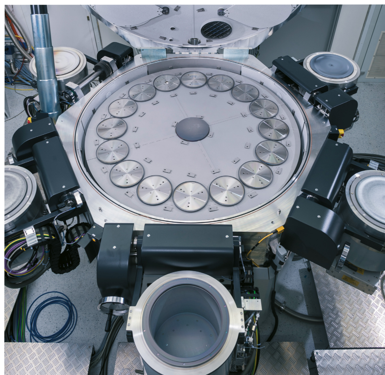
Figure 1a. Evatec CLUSTERLINE® 200 BPM deposition tool opened for service
