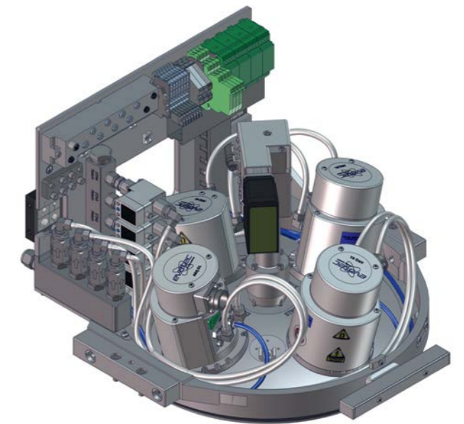
Figure 18: Drawing of the MSQ Multi-Source-Quattro with 3x sources DC/DC+ and 1x source RF/DC for co-sputtering and reactive sputtering of superconductive alloys.
