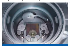
**Wire Feeder**Achieve thicker layers in e gun deposition
