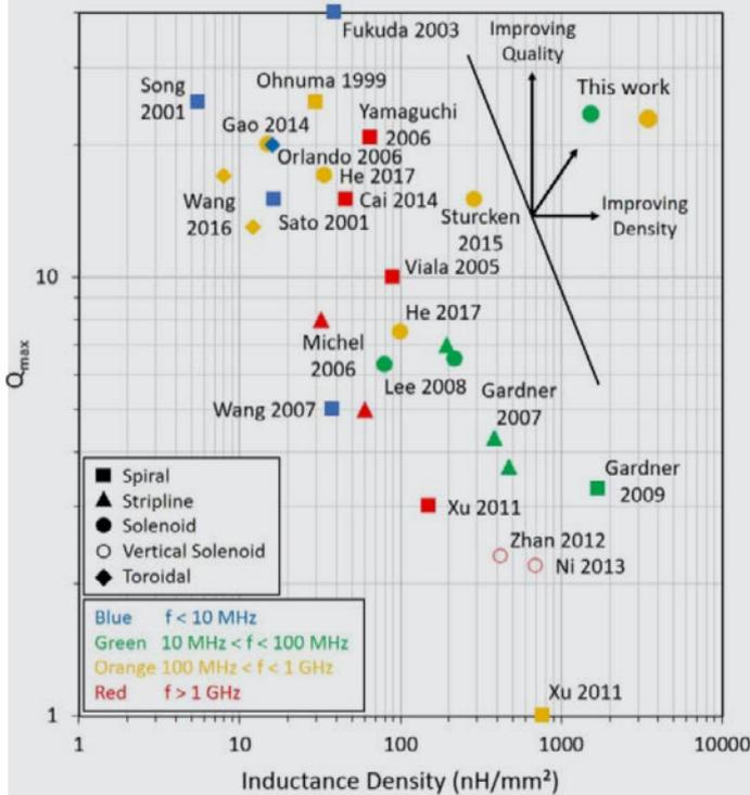
Figure 2. Peak quality factor versus inductance density of on-chip inductors from published measurements. The colours represent the frequency of the peak quality factor. – J.P. Michel et al., *IEEE Trans. Magn.* 55, 8401207 (2019)
