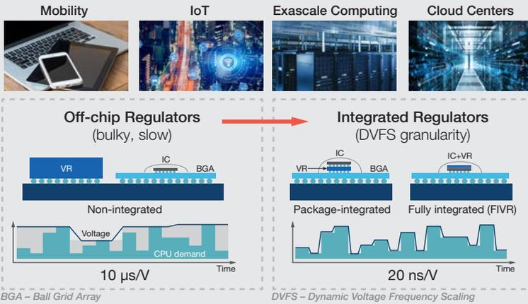
Figure 1. Evolution of Voltage Regulators onto the chip
