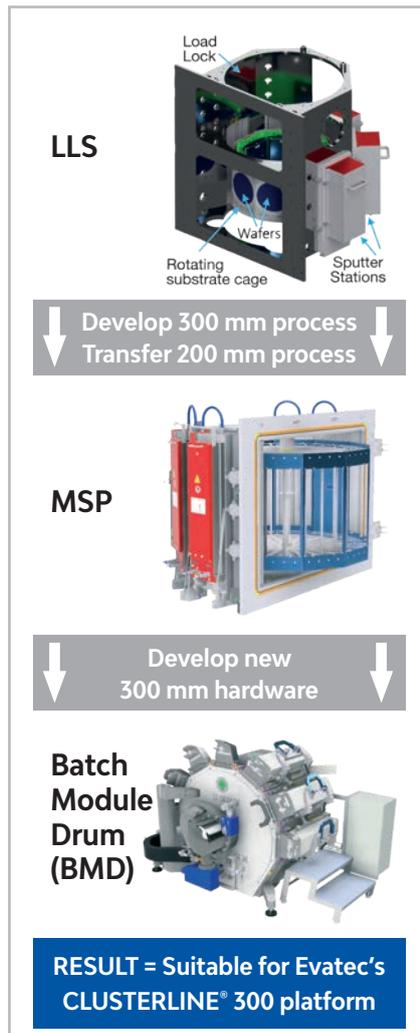
Figure 4. Development process of a new module
