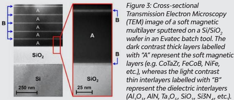
Figure 3: Cross-sectional Transmission Electron Microscopy (TEM) image of a soft magnetic multilayer sputtered on a Si/SiO<sub>2</sub> wafer in an Evatec batch tool. The dark contrast thick layers labelled with "A" represent the soft magnetic layers (e.g. CoTaZr, FeCoB, NiFe, etc.), whereas the light contrast thin interlayers labelled with "B" represent the dielectric interlayers (Al<sub>2</sub>O<sub>3</sub>, AlN, Ta<sub>2</sub>O<sub>5</sub>, SiO<sub>2</sub>, Si<sub>3</sub>N<sub>4</sub>, etc.).
