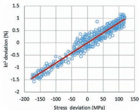
Figure 1. Deviation from average of the coupling coefficient as a function of Al<sub>0.7</sub>Sc<sub>0.3</sub>N thin film stress variation: the slope is steep and translates into 0.5% of coupling change every 50 MPa
