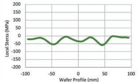
Figure 3. Within-in-wafer stress profile for an Al<sub>0.9</sub>Sc<sub>0.2</sub>N film deposited with the optimized process. The stress range is below ±50 MPa up to 5mm E.E.
