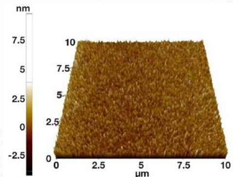
Figure 4. 10µm by 10µm AFM topography of an Al<sub>0.8</sub>Sc<sub>0.2</sub>N film deposited on Mo bottom electrode: the surface is free of abnormal grains.
