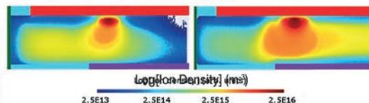
Figure 2. Plasma density obtained from simulations for two different RF-DC parameters: we can shape the plasma in order to obtain uniform ion bombardment.
