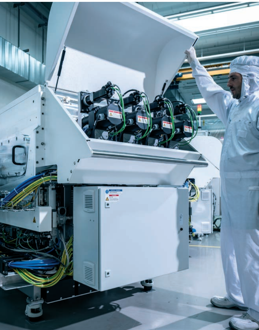
Figure 3. Rotating cathodes in PVD chamber
