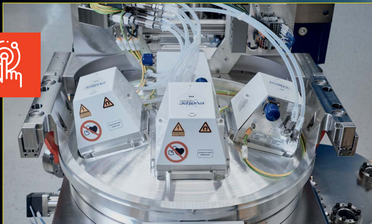
Figure 1: First demonstrator equipped with 4 FTC sources in the Evatec Competence Laboratory
