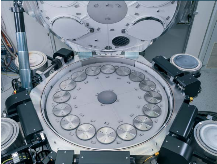
The latest generation of CLUSTERLINE® 200 BPM integrating a turntable with individual rotating chucks, proprietary cathode magnet technology and in-situ broadband monitoring.
